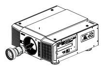
5. Secure the lens in the lens holder by turning counterclockwise the lens to the "locked" position.
