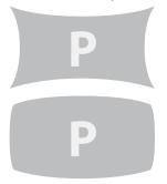
Press ◀ ▶ to correct pincushion distortion to correct image.
